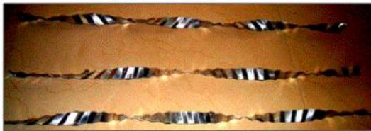
**Fig-3:** Actual view of wavy twisted tape inserts
